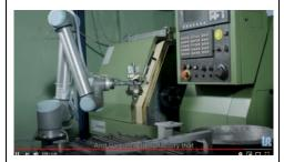
The use of Universal Robots within New Engineering Works heavily supported the loading and unloading of parts within the CNC machine. This thereby heavily contributed to reduced handling in the production facility.
