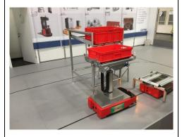
This AGV significantly reduces handling in production. KATE picks up small load carriers from a rack system in the warehouse and automatically conveys it to an intermediate store, so that employees just load their machine.
